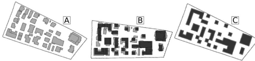
Fig. 3. The Generalisation process of buildings in a quarter: A) Original buildings; B) Rotated quarter and the generalised 10 meter rasterised buildings in red; C) Final result
