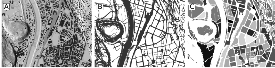
Fig. 1 A) Shaded landuse map of Trento and buildings; B) Non-nil pixel groups which split the city space into quarters (inverting pixel map); C) Final map of raw quarters (defining quarter areas having unique values)
