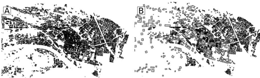
Fig. 8. 2D footprints depicted on final 3D scene: original buildings (left); generalised buildings (right). View direction – from right to left side of the picture
