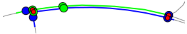
Figure 7. Segment of line A (city planning) – green; segment of line B (cadastral) – blue. Nodes of the most similar line segments with different lengths of segment: red points – l=41,i=5,j=5,G_Ind=2.35; green points – l=10,i=5,j=5 G_Ind=1.69; blue points – l=43,i=3,j=3 G_Ind=1.64.
